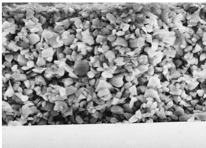
Electron microscope photograph of a cross section through a glass plate with silica layer (magnification x 500)
